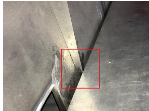
Figure 7. Pillar welding out of tool
